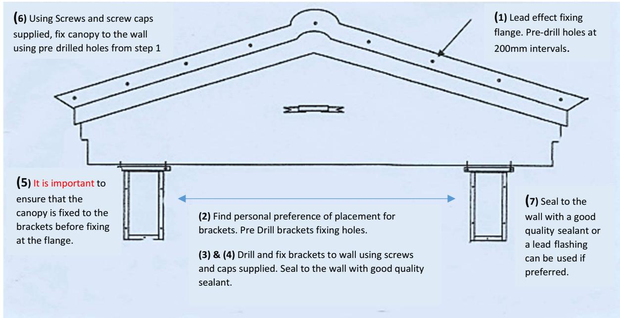
1. Mark out and pre-drill 6mm holes at approximately 200mm intervals along the canopy lead effect flange across the top of the canopy.
